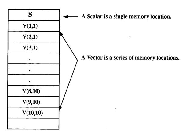
Cray research systems, like other computing platforms, have machine instructions that operate on scalars. However, unlike most other computers, the Cray systems also have machine instructions that operate on vectors.
