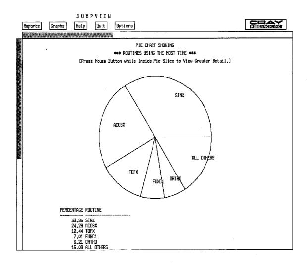
Notice first of all that the routine FAC is no longer present. From the **Flowview** analysis, it is clear that TofX, FUNC1 and PROD are the routines to optimize. The **Jumpview** analysis tells us that TofX and FUNC1 are doing most of the computational work
