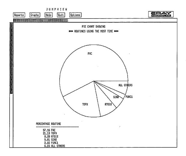
Notice first that the routine PROD does not appear in the **jumptrace** analysis, but it does appear in the **flowtrace** analysis. Very little CPU time is spent inside the routine PROD, it basically calls two orther routines. Notice that jumpview also reports on SIN% and RTOI%, computationally intensive system routines. Click on the pie slice FAC.
